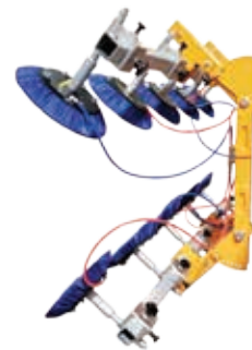
Vacuum cups and modified frame for curved glass
